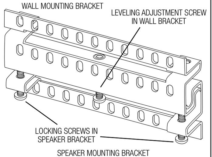
and bottom set of mounting holes on the rear of the speaker. Position the brackets similar to the ones mounted on the wall with the “J” bend up so it can hook into the wall bracket. Attach brackets to the rear of the speaker using four screws per bracket (Fig. 1 & 2).
