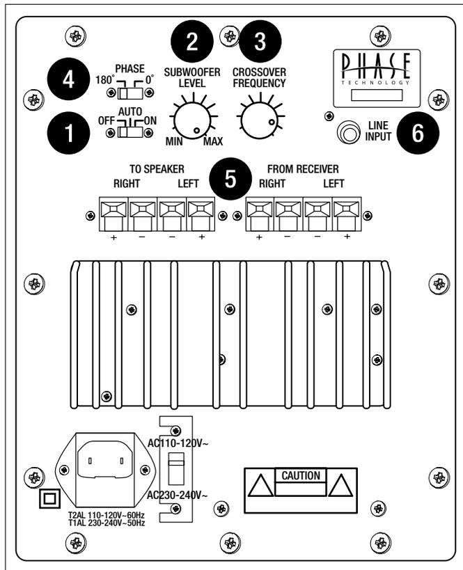
1. **Power ON/Auto/OFF:** This switch, when left in the “Auto” position, automatically activates the subwoofer when an audio signal is detected and shuts the subwoofer off after approximately ten (10) minutes of silence.
